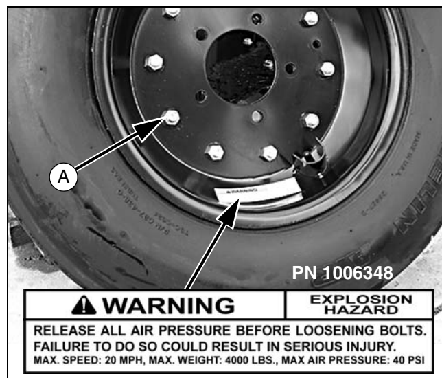
Figure 23. Split Rim Tire Servicing
